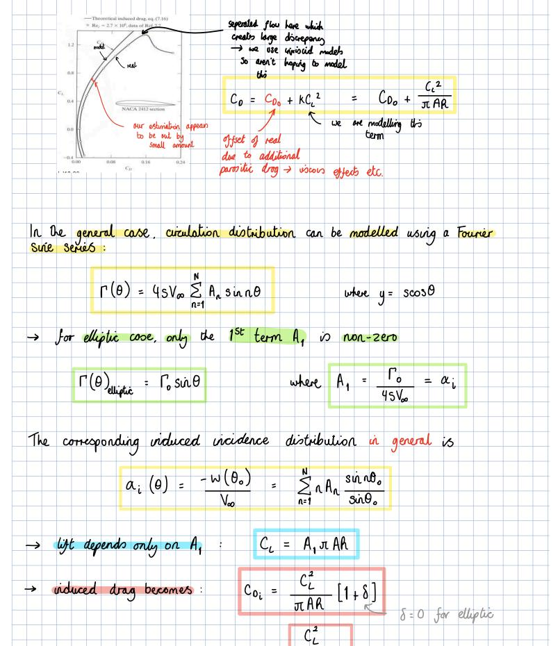
where  $e = \frac{1}{1+\delta}$  'span efficiency factor' e=1 for elliptic
