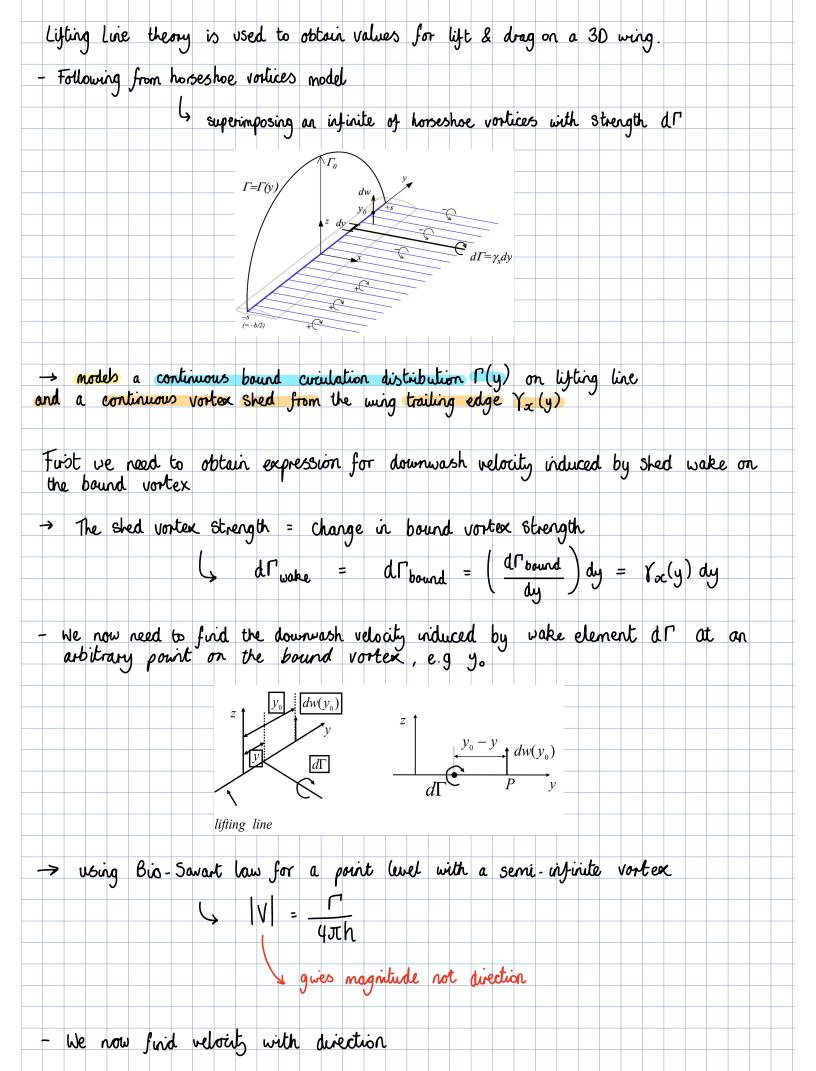
→ velocity viduced at y, by a filement y with +ve criatation has magnitude:
